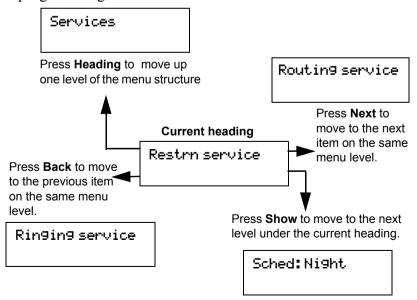
Programming buttons are active or inactive at different stages of programming. A button is active (meaning you can use that option), when the indicator next to it is lit ( $\triangleleft$  or  $\triangleright$ ).
