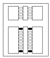
If you just want to cold start an individual module, on that module, simultaneously press the two top and two bottom buttons on the lower button set, as shown in the following diagram. The KIM displays a random pattern of icons as the KIM resets.
