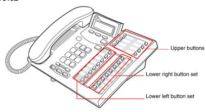
Line numbering starts on button 09 (default line assignments occur for DID, Hybrid and Square templates).
